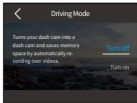
※ Driving Mode is available only in Video Mode and is disabled when the Code feature is set to H.265.
