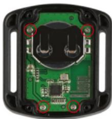
3. Lift the circuit board and slide out the battery, as shown below.
