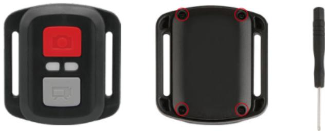
2. Remove another 4 screws on the remote's circuit board.
